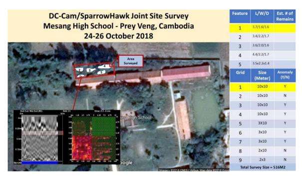
Displaying GPR's scanning results of sub-surface
